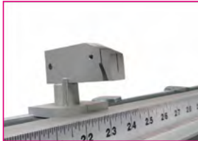
The handler has 2 adjustable blades, so you can cut two or three jobs at once.
