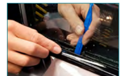
The tapered tail is quite stiff, yet flexible enough to push rubbers away from windows and other vehicle body parts. Because it is tapered and very smooth, it is a great tool for positioning windows before the water is squeegeed out from behind it.
