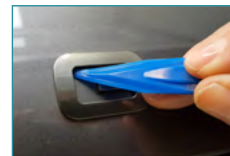
The curved tip tapers off and is ideal for pushing into corners and giving just that little bit of extra pressure to the rear side of edges, panels, doors etc.
