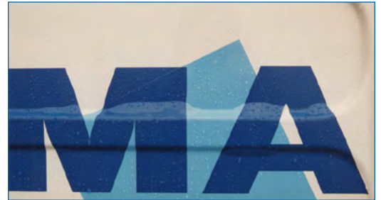
Due to the silicone content in modern car lacquers the adhesion of can be far from optimal. under tension (especially in recesses) is bound to come loose and ultimately be returned for repair or renewal.
