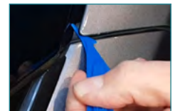
The curved tip tapers off and is ideal for pushing into corners and giving just that little bit of extra pressure to the rear side of edges, panels, doors etc.
