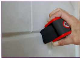
In this image you can see that the hard foam wheel easily takes the shape of the curved surface.
