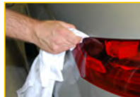
Simply take a squeegee and wrap a cloth around it. This will make the cleaning and degreasing of these hard-to-access areas a lot easier.
