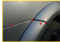
Good application is dependent on good adhesion. That goes without saying. Unfortunately, the cleaning and degreasing of the most critical areas get overlooked. These include joints, sills and gaps in bodywork. This is exactly where the tends to come loose and curl.
