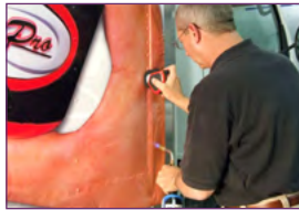
Warm up the and roll RollePro simply over rivets channels, grooves or joints.
