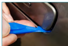
The Factotum II saw some improvements over version I. The tip tapers off and has a sharper edge. It is stiff, yet flexible. This allows a lot of force to be applied when pushing into the smallest of channels and creases, but it won't break.
