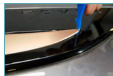
The Factotum II saw some improvements over version I. The tip tapers off and has a sharper edge. It is stiff, yet flexible. This allows a lot of force to be applied when pushing into the smallest of channels and creases, but it won't break.
