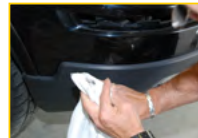
Ultra Clean cloths area ideal for checking to see if you have cleaned and degreased properly. These perfectly white cloths will soon show if any dirt is left in those awkward corners before you start application.
