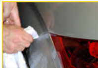
Thorough cleaning of any joints or other awkward areas is essential for good adhesion.
